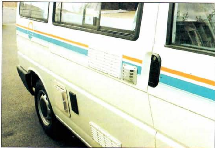
Offside: Cascade water heater flue, electrical hook-up, fridge vents and fridge flue.
