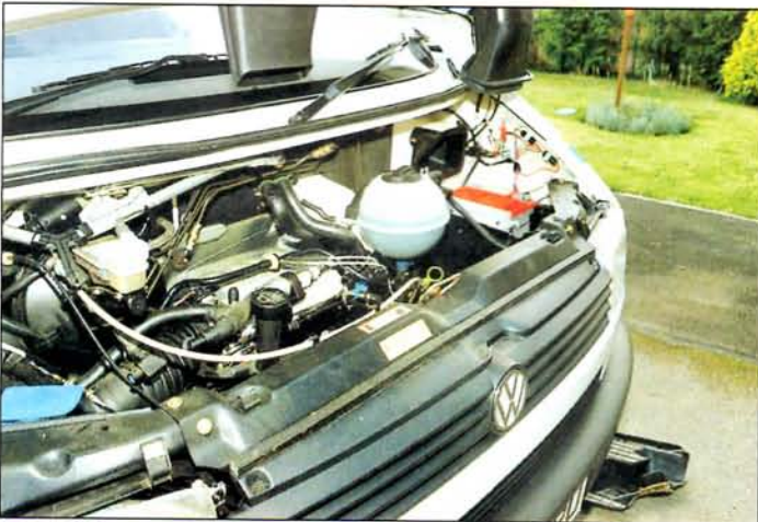
Beneath the bonnet. Twin batteries (right) have removable cover. Note fresh air scoop (central).
