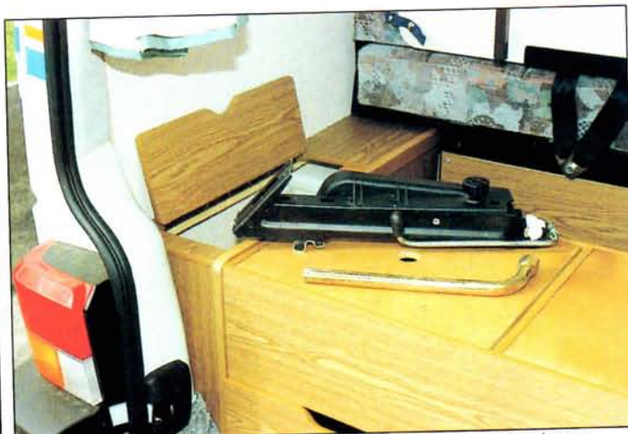
Side lift jack clips beneath sills for use, is stored with wheelbrace in locker shown.
