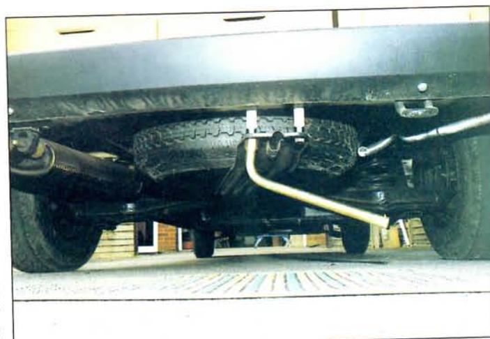
Two long bolts hold the spare wheel cradle and are operated with the wheelbrace as shown.
