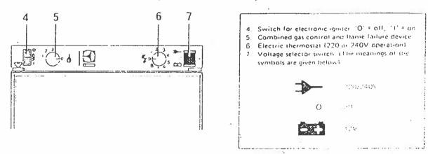
See that the voltage selector switch (7) is set at "O", i.e., is at its central (OFF) position.
